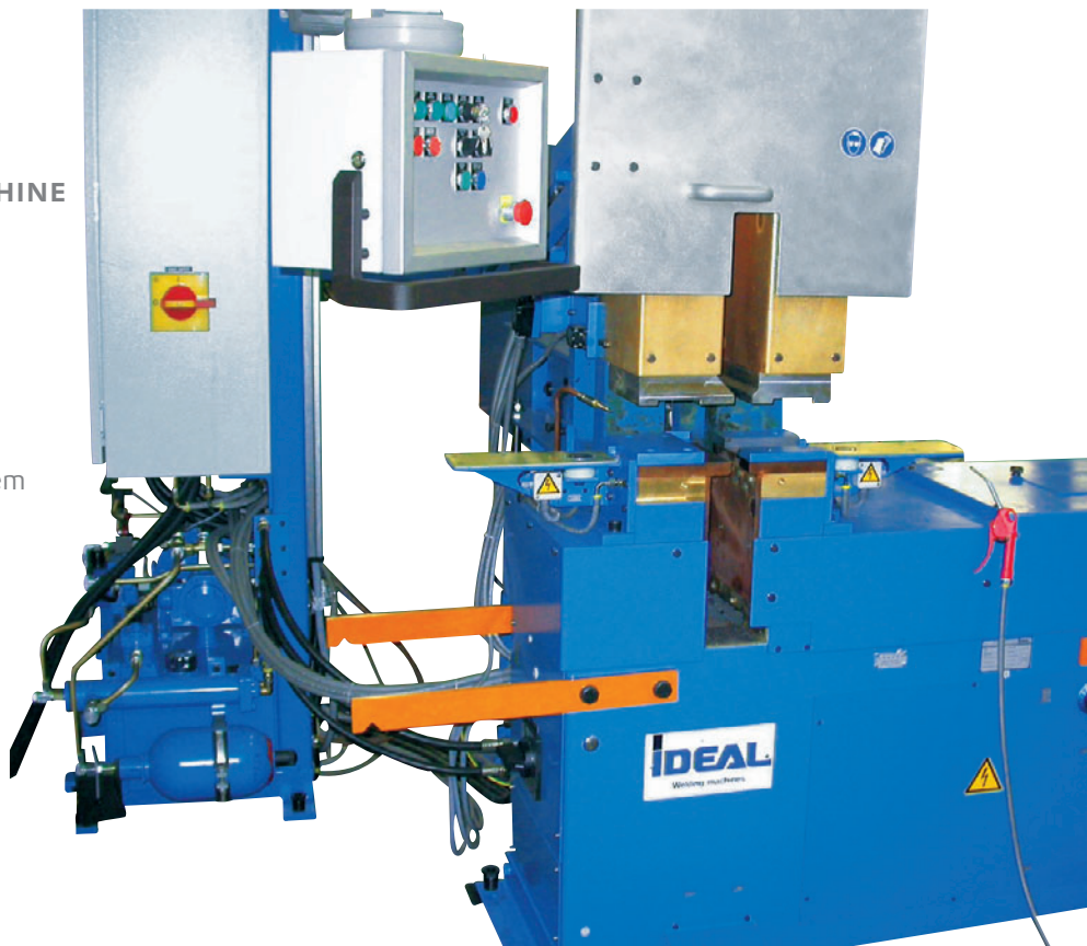
Type AS 40 for T-welding of rectangle tube
