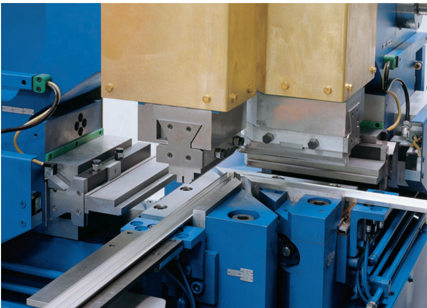
Mitre welding of aluminium frames
