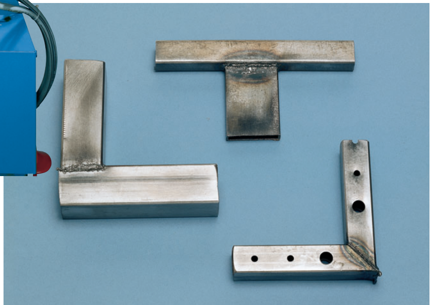
Tubular frames: butt, mitre or T-welding
