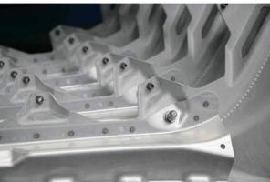
On each vehicle door, the professionals at GF weld 16 spots, each exactly 5 mm in diameter, in an approximately 100 sec cycle.
