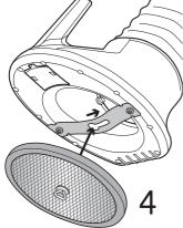
Ensure that the spark protection is pressed up against the hood with no gaps around the edge after mounting.
