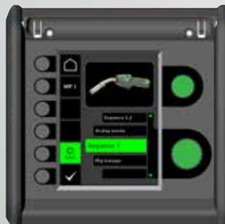
Choice of torch in the main menu; The Galaxy supports all MIG-A Twist torch functionalities
