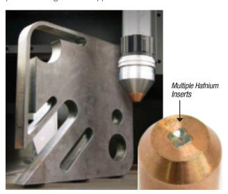
HeavyCut Technology Cuts Cost By Length on Mild Steel
