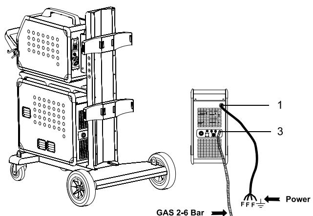
Important: stretch out welding hose, earth cable and interconnecting cable, as necessary, as shown in the figure to avoid affecting the welding performance and at worst destroying the welding machine.
