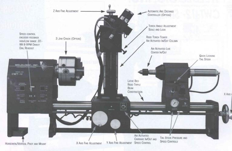
The Weldlogic CWT-12- Horizontal/ Vertical circumferential weld positioners are engineered to be a highly versatile, precision welding positioner. Our CWT wasn't adapted, but was specifically designed for precision automatic welding. Accuracy and repeatability permit circumferential, longitudinal and spot welds to be made automatically with a minimum of operator skill.
