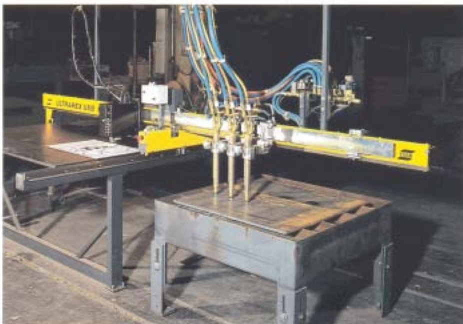
ULTRAREX UXB with three manually adjustable single machine cutting torches for simultaneous use in batch production
