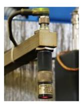
The laser pointer is attached to the support and shows its position above the work piece. It is a tool to align and position the torch above the plate, e.g. for edge starts. In the opposite case (machine stands still), it can be used as optical stopper, e.g. for plate alignment. Crosses are projected via a laser diode with a red light and a wavelength of approx. 635 nm. The applied laser equipment complies with laser class 2M and can be used without special safety requirements.
