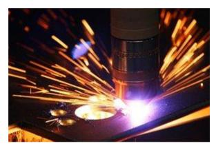
The Hypertherm HPR 400XD HyPerformance plasma cutting unit has the patented *True Hole technology* to align and focus the plasma arc, improving arc stability and energy for more powerful precision cutting.
