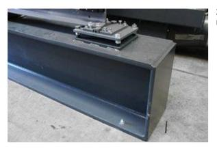
2 Pcs HEB450 profiles are supplied for the foundation of the machine track.
