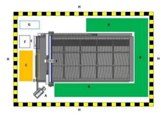
A – Control panel and orientation of the keypad and screen
