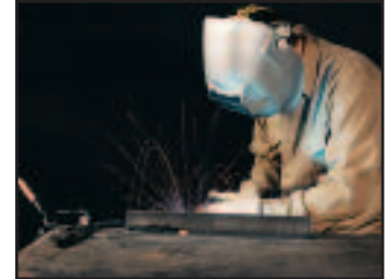
STT® using CO 2 and .045" solid wire. Note reduced spatter and fume.
