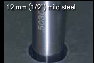
12 mm (1/2") hole without True Hole technology
