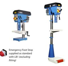
This floor or bench mounted drill incorporates a built-in low voltage worklight and table adjustment by rack/pinion mechanism. An integrated kick-stop switch is fitted to the front of the floor-mounted machine which is wired into a no-volt/overload release starter. A separate 'mushroom' style stop switch is supplied with the bench-mounted model ready for fitting on installation.
