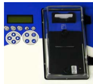
Operator panel with integrated printer and chip card manager for weld procedure transfer and storage
