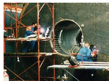
PS 254-2 power source with TS type tube sheet weld head
