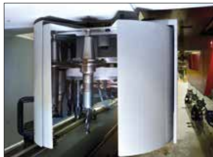
Automatic tool changer with up to 24 tools per drill head (depending upon the model)
